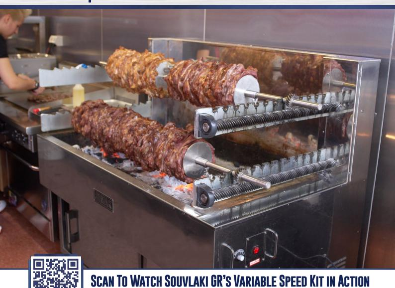
The Variable Speed Kit optional accessory for our M28C Series Charcoal Rotisseries allows you maximum control over the cooking process by seamlessly stepping down the motor from 11 to 3 RPM.
